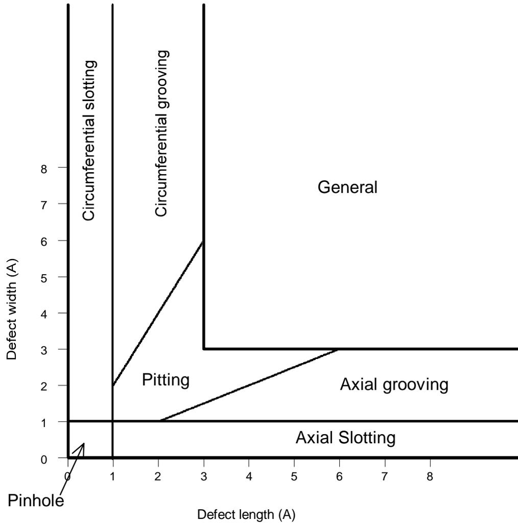
Figure 2: Graphical presentation of metal-loss feature type definitions
