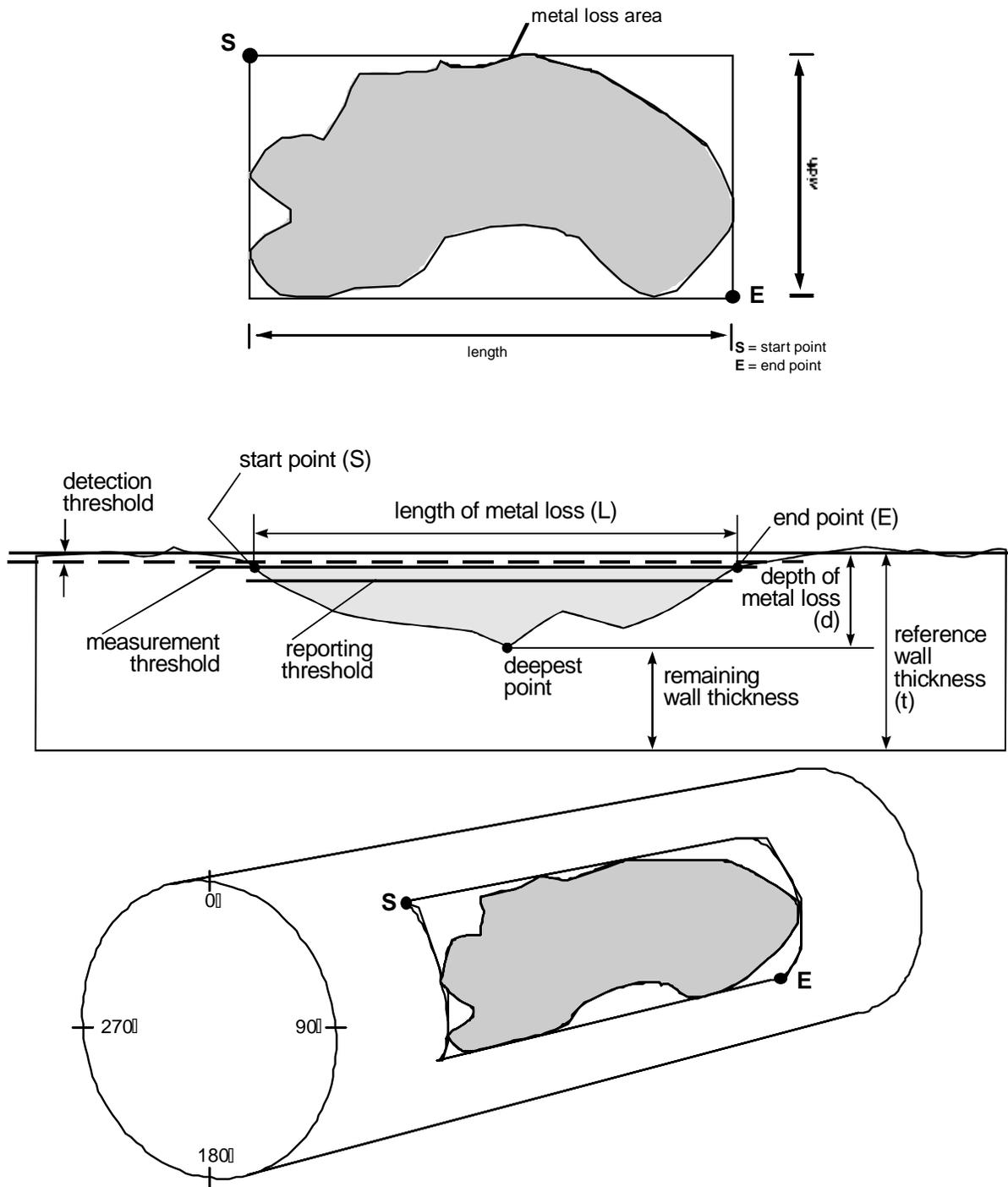
Figure 1: Location and dimensions of metal-loss features
